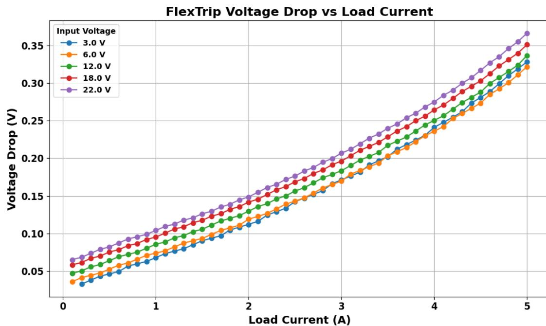
For the Protect Nano, the curves of interest would be the 3, 6, 12 V operating curves corresponding similarly to the 3.3, 5 and 12 V modes of operation.
