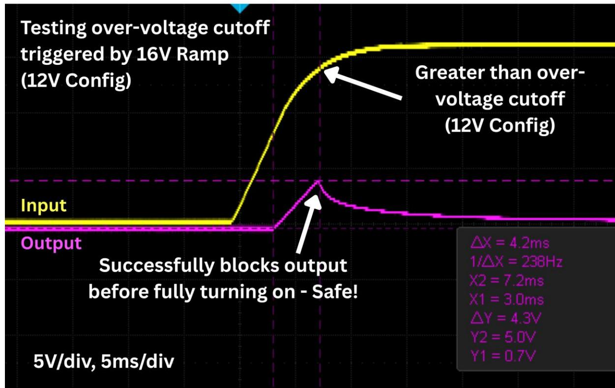
As can be seen, when the 13.5 V OVC threshold is exceeded in 12 V mode, the turn-on processed is paused and the voltage falls from its peak value at 5.0 V, so the downstream devices never see this 16 V setting that otherwise would have been applied!
