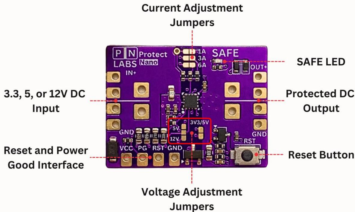
To set up the Protect Nano module for **protection operation**, do the following:
