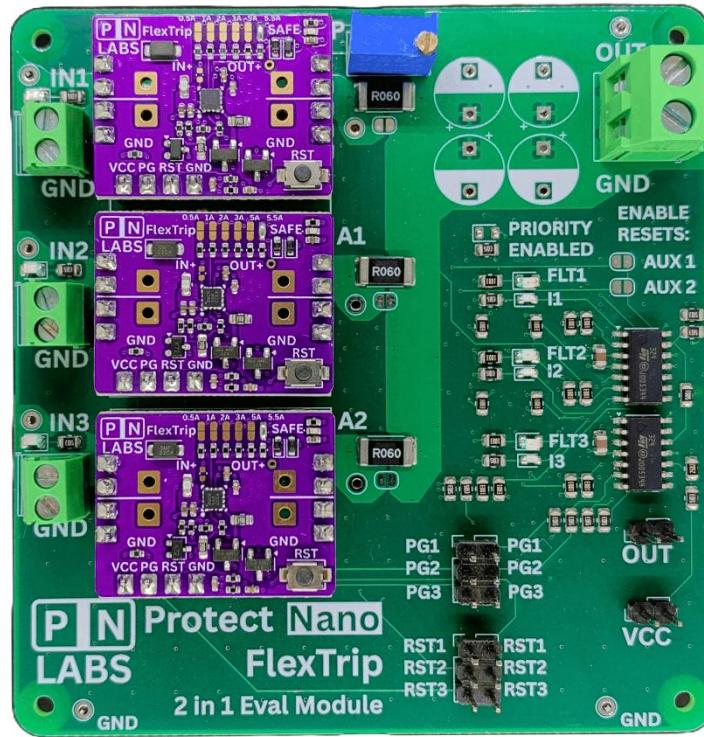
This configuration isolates the power paths by virtue of the internal ideal diode to the Protect Nano IC. Both paths should share the current equally if the input voltages are the same, with current sharing ceasing if the voltages have a difference greater than ~0.6 V.
