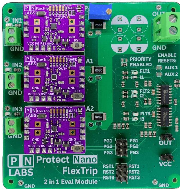
This configuration isolates the power paths by virtue of the internal ideal diode to the FlexTrip IC. Both paths should share the current equally if the input voltages are the same, with current sharing ceasing if the voltages have a difference greater than ~0.6 V.
