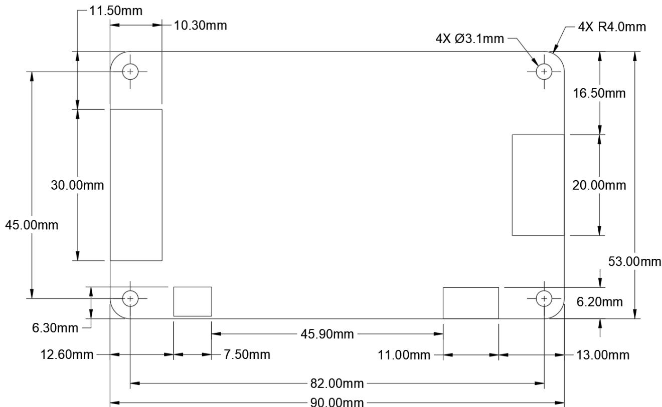
The height from the bottom of the FR4 to the tallest component is 15.85mm.
