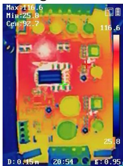
17V input 12V @ 10A + 5V @ 5A + 3.3V @ 5A resistive loads ran continuously for 10 minutes:
