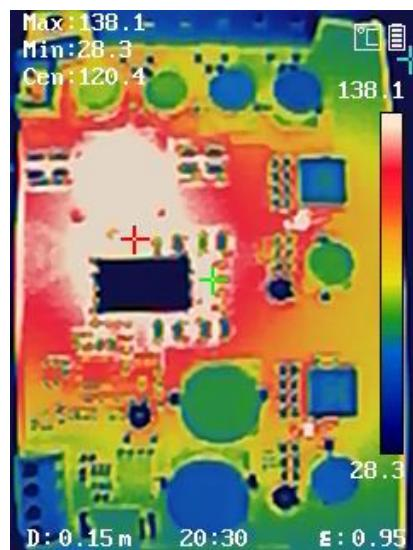
24V input 12V @ 10A + 5V @ 5A + 3.3V @ 5A resistive loads ran continuously for 10 minutes:
