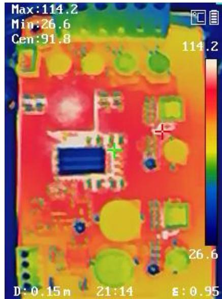
As can be seen in the tests, the Power Pal never reaches beyond 120 C for high loads at 17 and 24 V input, and stays below 140 C at the max input voltage (52 V).
